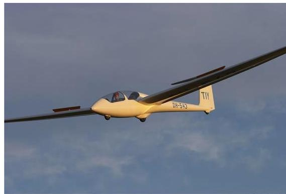
ASK-21 on final approach, before “roundout” or flare to land on main and tailwheel. Use about 1/2-3/4 airbrake, 55-60 knots.
